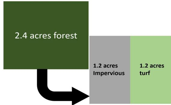
Figure 3. Land use conversion implemented in SWMM in each scenario subbasin.
