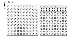
**Figure 3.** The grid used for the numerical solution with the conventional approach (left) and component-based approach (right)
