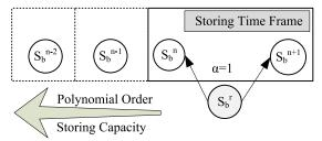
Figure 5. Provided interpolation routine in OpenMI which allows for linear interpolation (when  $\alpha = 0$ ), nearest neighbor (when  $\alpha = 1$ ), and a weighted approach between these two alternatives (when  $0 < \alpha < 1$ )
