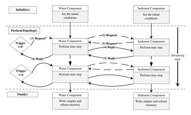
**Figure 7.** Communication flow for a bidirectional link within OpenMI between the water and sediment components (adapted from *Sinding et al.* [2005]).
