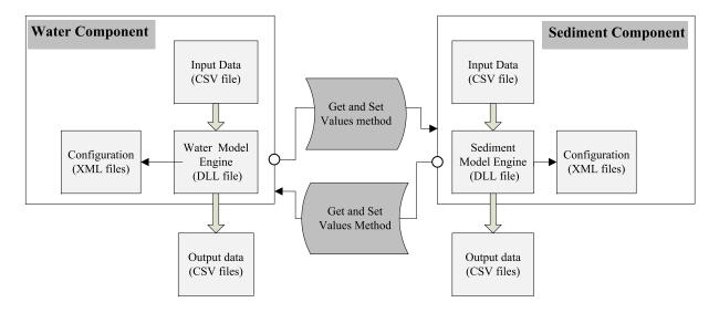
Figure 4. Details for the implementation of the component-based model approach.
