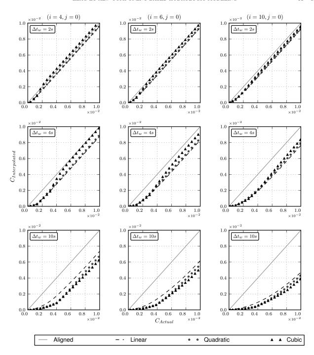
**Figure 9.** Results of linear, quadratic, and cubic spline schemes in minimizing the mass balance error between temporally misaligned coupled components. Comparison is for three locations in the sediment top layer (x = 4, 6, and 10 m) and for three values of internal time step differences (2, 4, and 10 s).
