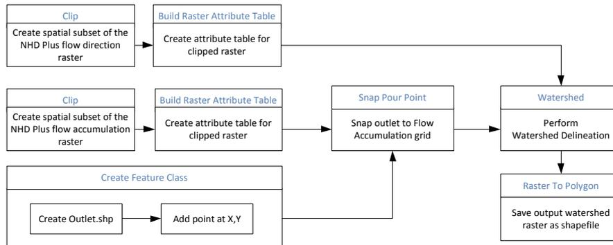
Figure 7: The procedure used for watershed delineation using ArcGIS tools, automated using the Python programming language.
