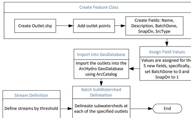
Figure 10: The procedure for subwatershed delineation within ArcGIS, using Arc Hydro Tools.
