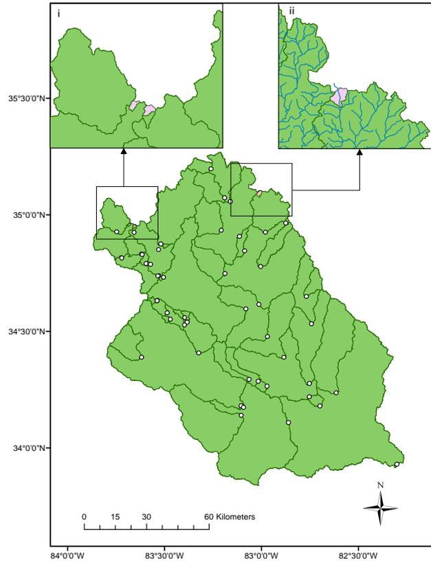
Figure 11: *Subbasins were delineated at USGS streamflow stations using Arc Hydro Tools and the hierarchical approach. Boundary differences were found when compared with raster-based delineation and are illustrated by the lighter catchments in insets (i) and (ii).*
